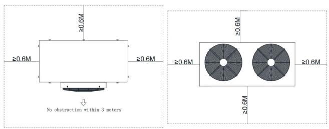
Figure 2-4 Recommended installation spacing diagram for unit installation
