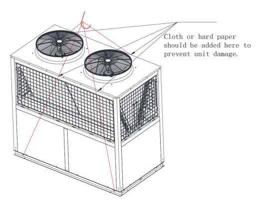
Figure 2- 3 Lifting of the unit
