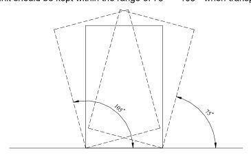
Figure 2-1 The tilt angle of the unit
