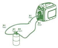
Tank Cooling Procedure in the recovering process.
